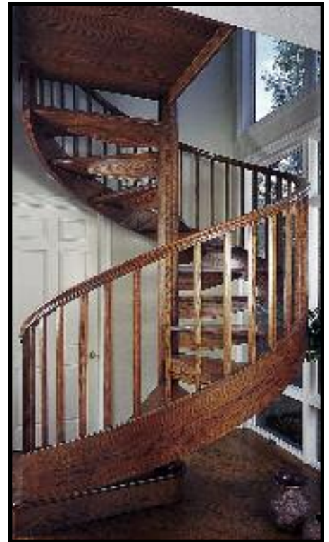
76AW #240 oak rail, #334 balusters, custom stringer and starter step
